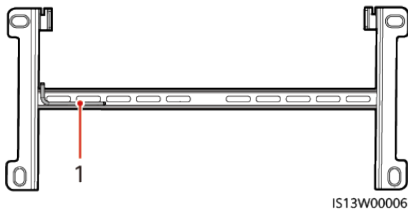
Figure 4-9 Position for binding the torx key
