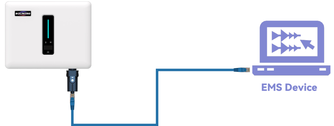
Method 1. Connect the DuoCOM to the EMS device directly
