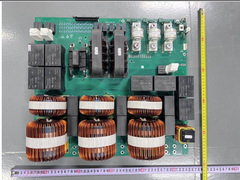
Figure 23. M2, AC/DC power board– front
