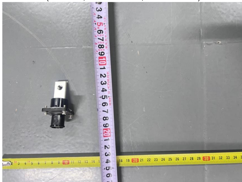
Figure 8. Dc terminal - (for model , TAA-105KW-11,TAA-125KW-11)
