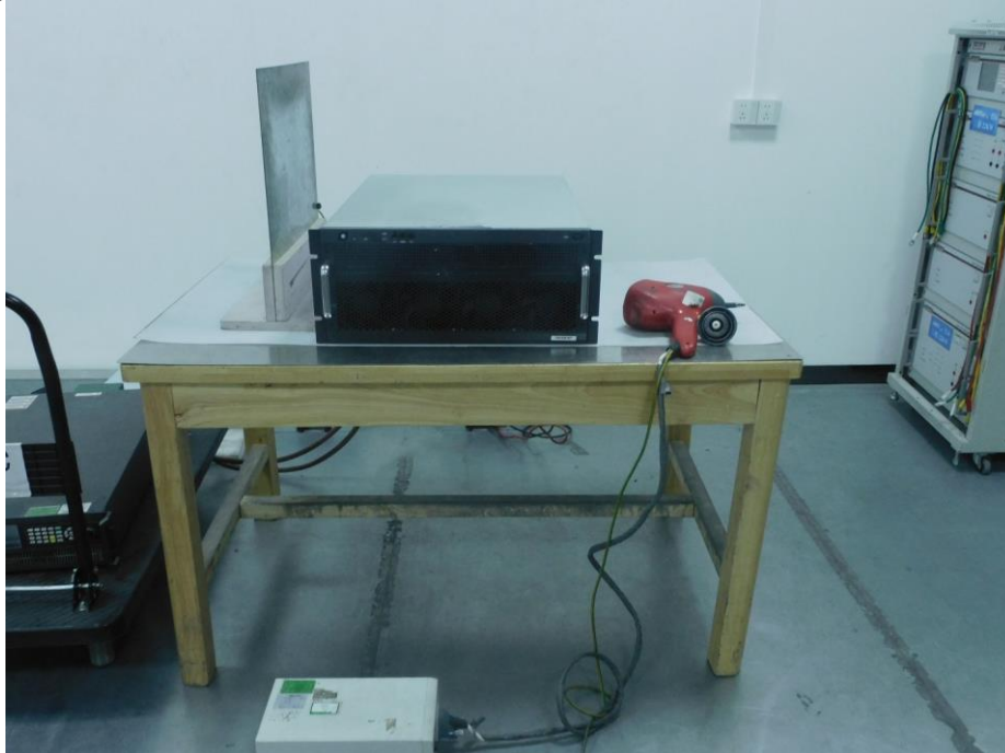
Photograph 9: Set-up for Voltage Dips and Interruptions
