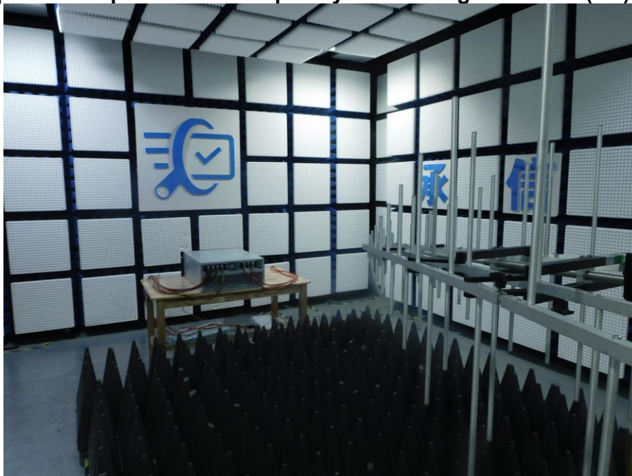
Photograph 3: Set-up for Radio Frequency Electromagnetic Field (RS)
