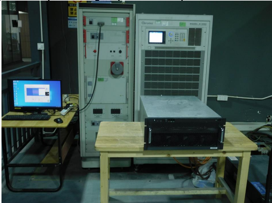
Photograph 9: Set-up for Voltage Dips and Interruptions
