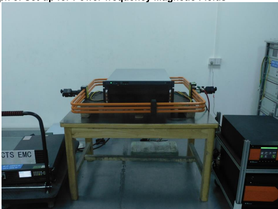
Photograph 5: Set-up for Power-frequency Magnetic Fields
