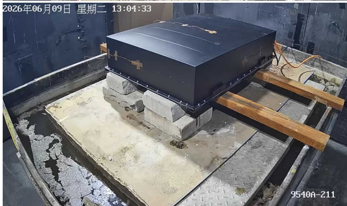
1 st cell thermal runaway induced [13:04].
