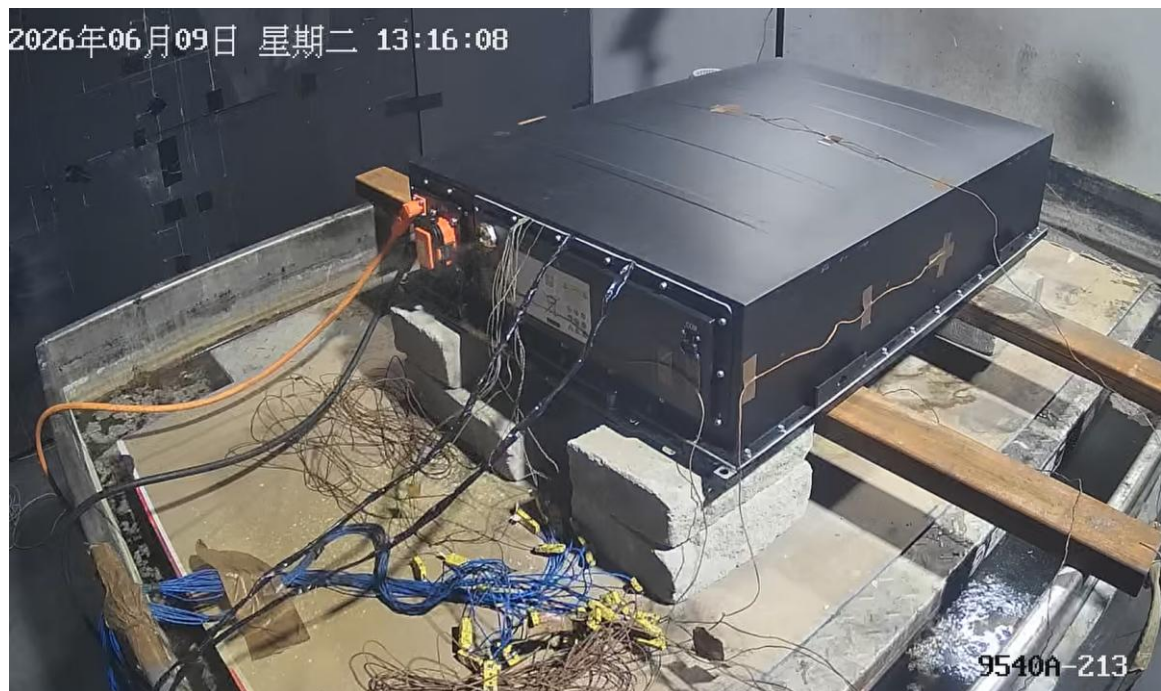
2 nd cell thermal runaway induced [13:16]
