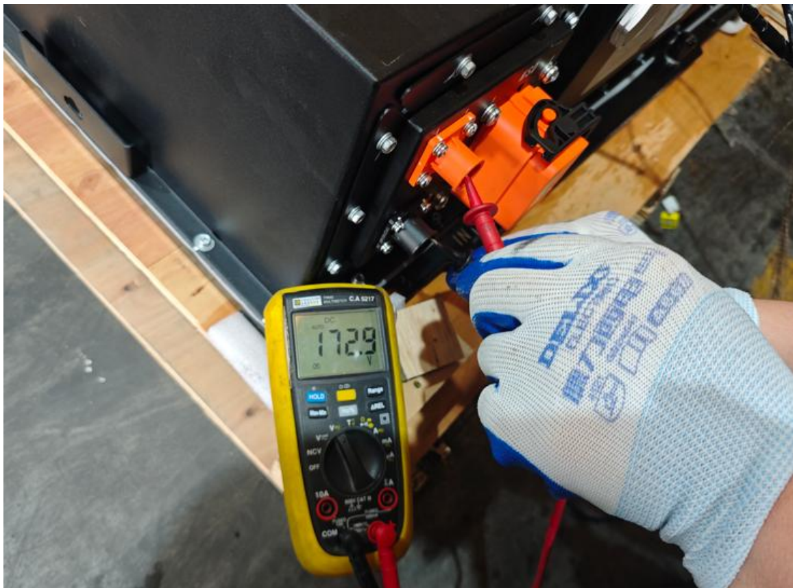
Module voltage before test [172.9 V]
