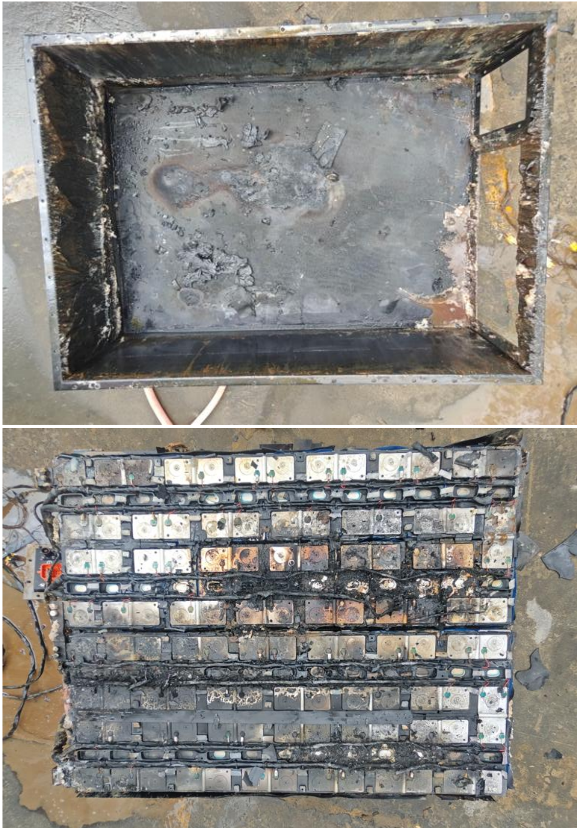
Internal view of the initiating module after the test
