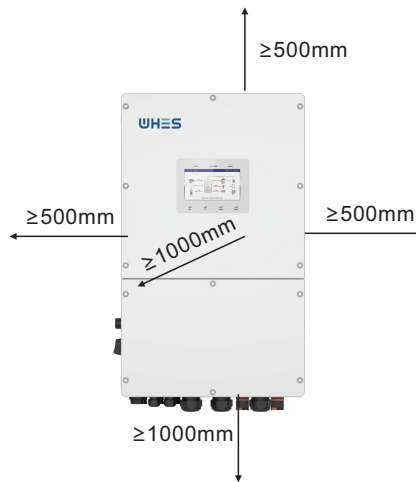
Figure 3.5 Inverter Mounting Clearances
