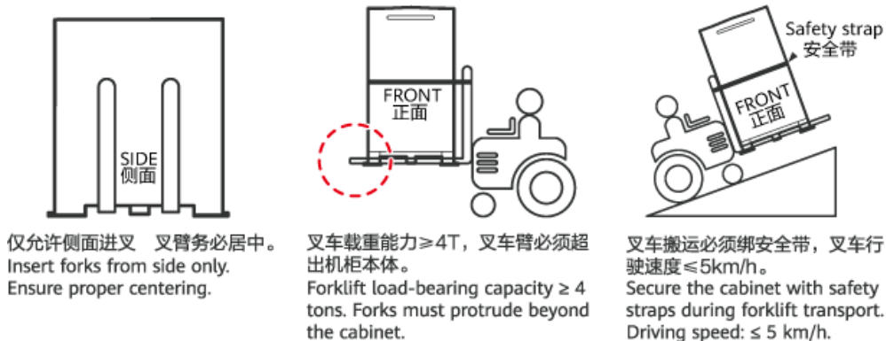
Figure 3-1 Loading and unloading requirements
