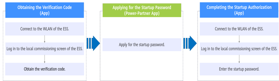
Figure 9-2 ESS startup authorization procedure
