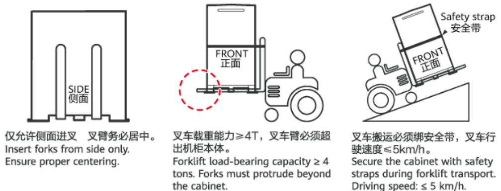
Figure 3-1 Loading and unloading requirements
