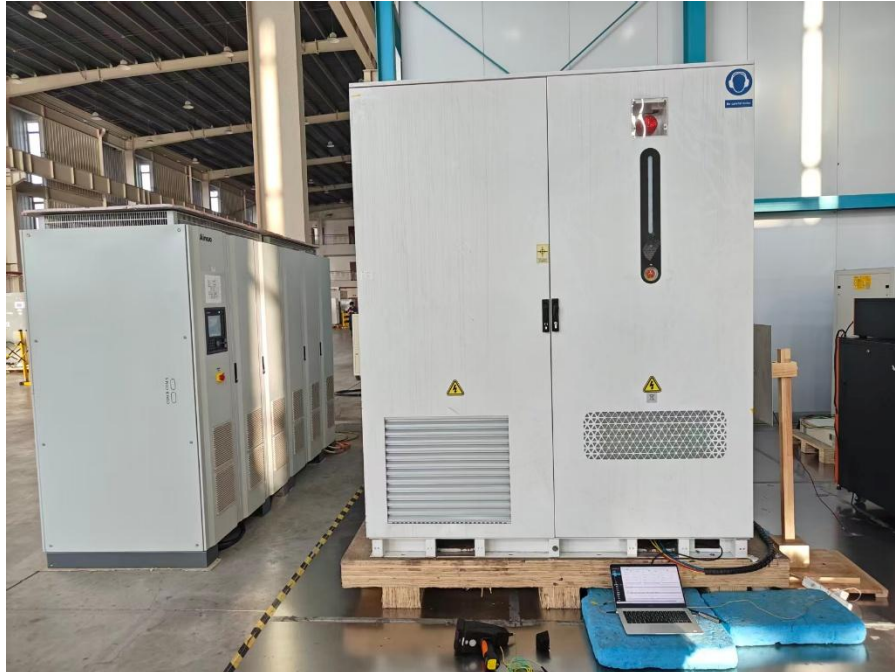
Photograph 3: Set-up for immunity test of electrostatic discharge
