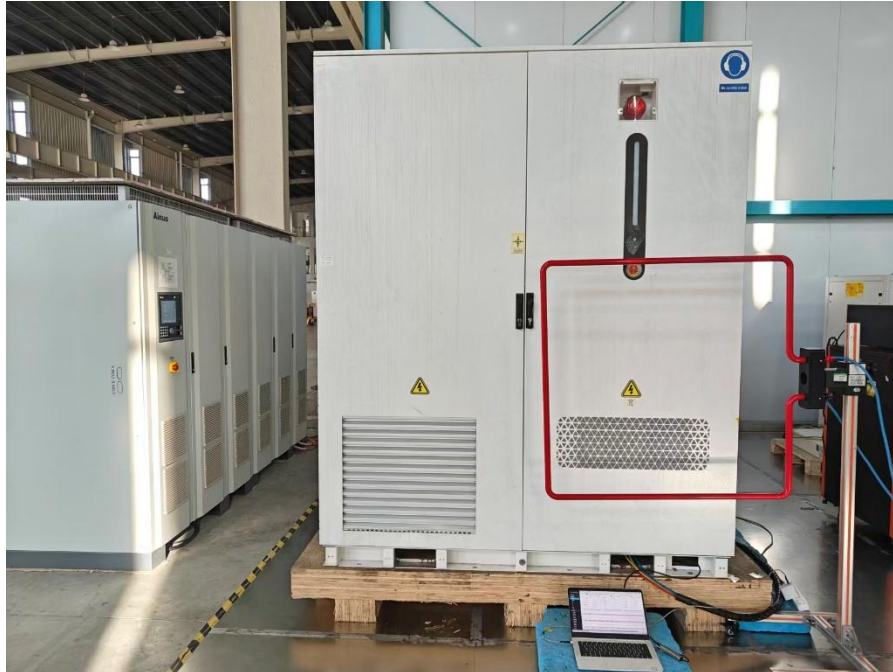
Photograph 5: Set-up for immunity test of power-frequency magnetic field
