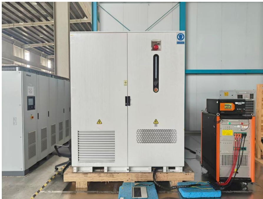
Photograph 6: Set-up for immunity test of fast transients
