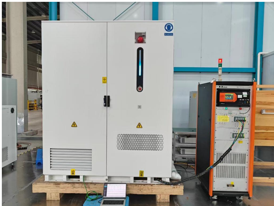
Photograph 6: Set-up for immunity test of fast transients
