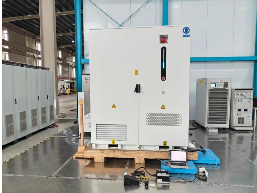
Photograph 3: Set-up for immunity test of electrostatic discharge
