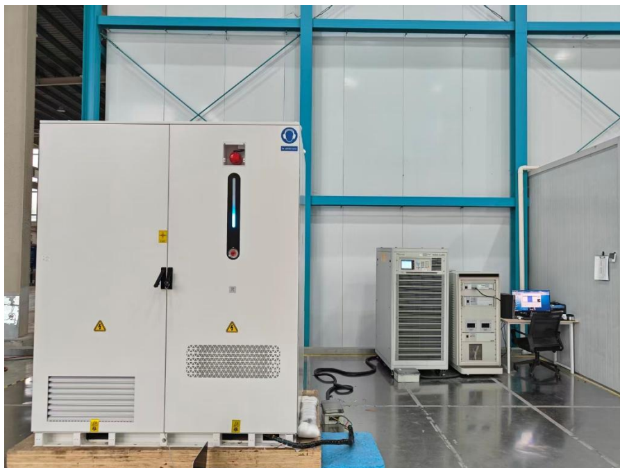
Photograph 9: Set-up for immunity test of voltage dips and interruption
