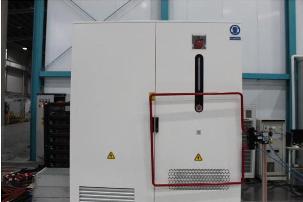
Photograph 5: Set-up for immunity test of power-frequency magnetic field
