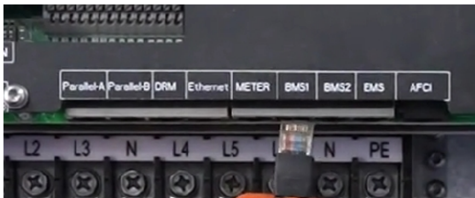
Figure 7- 17 Inverter Bottom BMS Interface
