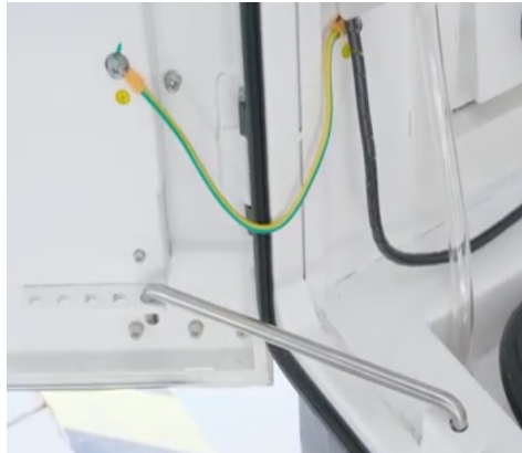
Figure 7- 10 Door stopper position
