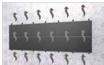
Very good rear ventilation of the modules
