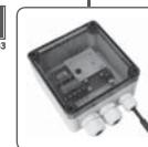
TEV-2 Thermostat for regulation of heating (cooling), adjustable range -20 to +20 °C (-4 °F to +68 °F), externi sensor NTC, external sensor NTC, output contact 16A changeover/SPDT.
