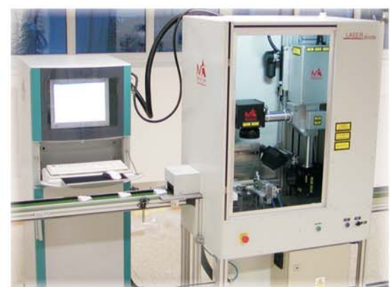
12) In the end the products are fully printed by laser technology. Laser can burn from upper part) side of the product) and side part (front panel and terminals) printing one piece takes about 30 s.
