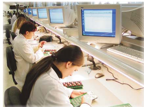
9) After necessary semi-product testing on pin-testers (Pic.9) final assembling into enclosures is executed. The actual state of completion is monitored by bar codes during the whole production process (Pic.10).
