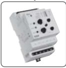
TER-4 Wide and accurate range of setting -40 °C to +110 °C (-40 °F to 230 °F) in ten ranges in one device, fine temperature setting. 2 inputs for NTC sensor, 2 outputs 16 A changeover/SPDT, additional function (memory, hysteresis, indication of faulty sensor). Supply: AC 230 V or AC/DC 24 V (galv. separated).
