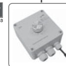
TEV-3 Thermostat for regulation of heating (cooling), adjustable range +5 to +35 °C (41 °F to 149 °F), external sensor NTC, output contact 16 A, control potentiometer and indication on panel.
