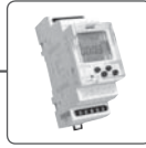
TER-9 Digital multifunction thermostat 2 temperature inputs, 2 outputs 8A changeover/SPDT, 6 functions, in-built time switch clock, LCD with back light, galvanically sep. supply voltage AC 230 V or AC/DC 24V, 2 MODUL. Temperature range: -40 °C to +110 °C / -40 °C to 230 °F
