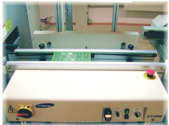
4) PCBs with mounted SMD components are inspected and forwarded to reflow.
