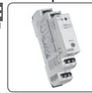
TER-7 Monitoring heating of motor winding in range given by resistance of in-built PTC thermistor (1.8-3.3 kΩ), additional function (memory, reset), output contact 2x8A changeover/SPDT, supply: AC/DC 24-240 V.
