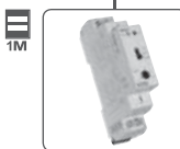
CRM-42F programmable staircase switch without warning before switching off, time setting by number of button pressings.
