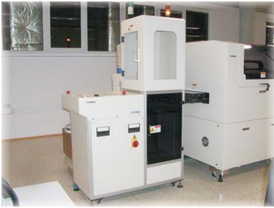
1) Printed circuit boards are placed into a cartridge and then automatically delivered to SMD production line.
