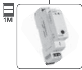
CRM-81J 3 functions and 6 time ranges, multivoltage or 230V supply, output 16A changeover/SPDT.
