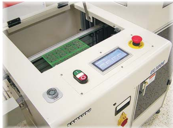
6) Fully automatic line is ended by a cartridge which distributes picked and cured PCBs into holders.
