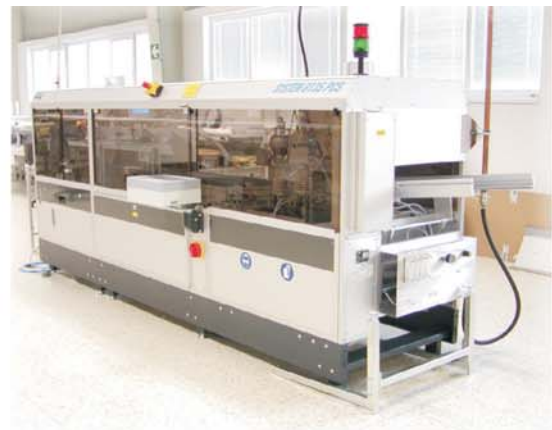
8) Manual placing of classical components is followed by soldering in soldering unit SEHO 8135-PCS which already supports "lead free" soldering technology. Thanks to IR pre-heating, this soldering unit allows operations on PCB together with temperature sensitive components on the upper side of PCB. Soldering unit is equipped by LW soldering jet and Delta jet. These jets allow a good quality.
