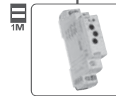
CRM-61 cost effective version of CRM-91H, 6 functions, 6 time ranges. Output 8A changeover/SPDT, supply AC 24-240V, DC 24V.
