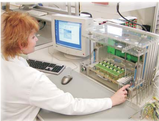
9) After necessary semi-product testing on pin-testers (Pic.9) final assembling into enclosures is executed. The actual state of completion is monitored by bar codes during the whole production process (Pic.10).
