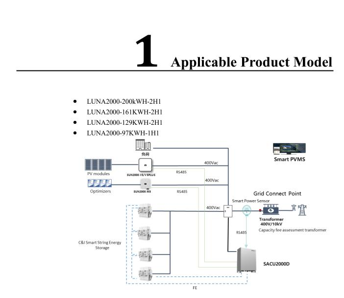
Huawei C&I Smart String Energy Storage (ESSs for short) Products LUNA2000B series are applicable to industrial and commercial scenarios. They work with the SmartPCS, DCDC and SACU. The SmartPCS is connected to the pack controller DCDC, and charges battery when the power grid is sufficient. When the power grid needs to be output, the SmartPCS outputs the stored battery energy to loads for use.
