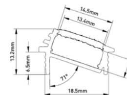
Cut-out width: 18 - 18.2mm Depth: 6.7 - 7mm
