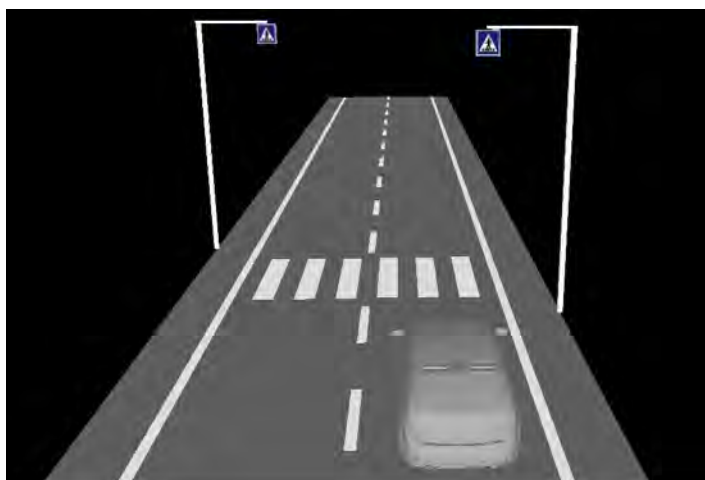
Vizualizácia umelého osvetlenia priechodu pre chodcov so svetidlami Zebra Sign. (Visualization of artificial light pedestrian crossing lamp Zebra Sign.)
