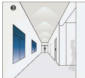
After a period of time when the micro sensor does not detect any further movement, the luminaire will revert to 10% light output as standard
