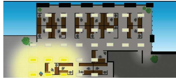
2. As people enter, lighting in their area dims up to "task level." Others in the group dim up to "background level."
