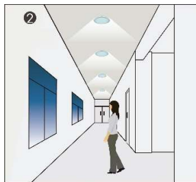
When movement is detected by the in-built micro sensor, the luminaire increases its output to 100%
