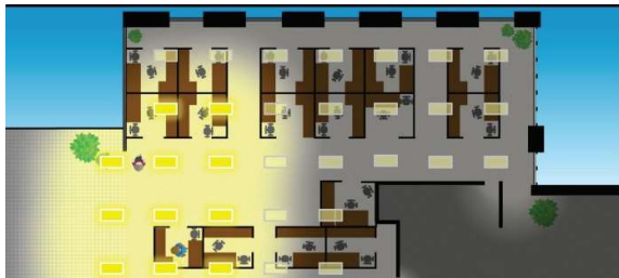
3. As additional people enter, lights in their area dim up to "task level."
