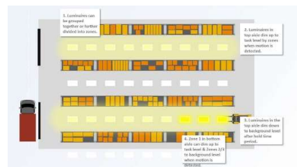
4. Zone 1 in bottom aisle can dim up to task level and Zones 2/3 to background level when motion is detected
