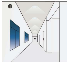
The luminaires stay at 10% light output
