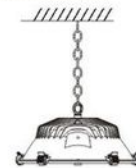
Hanging chain installation
