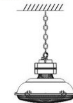
Hanging chain installation
