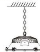
Hanging chain installation
