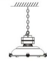
Hanging chain installation
