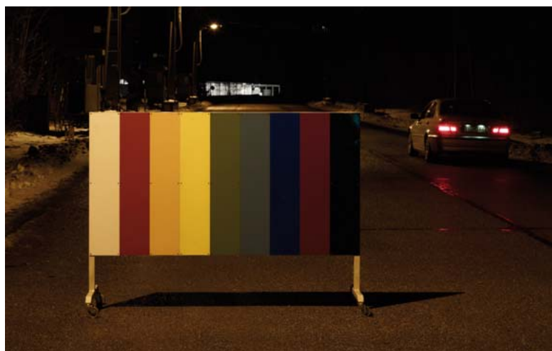
HST – road and surroundings have a yellow tinge. Color rendering is poor. R_a < 40
