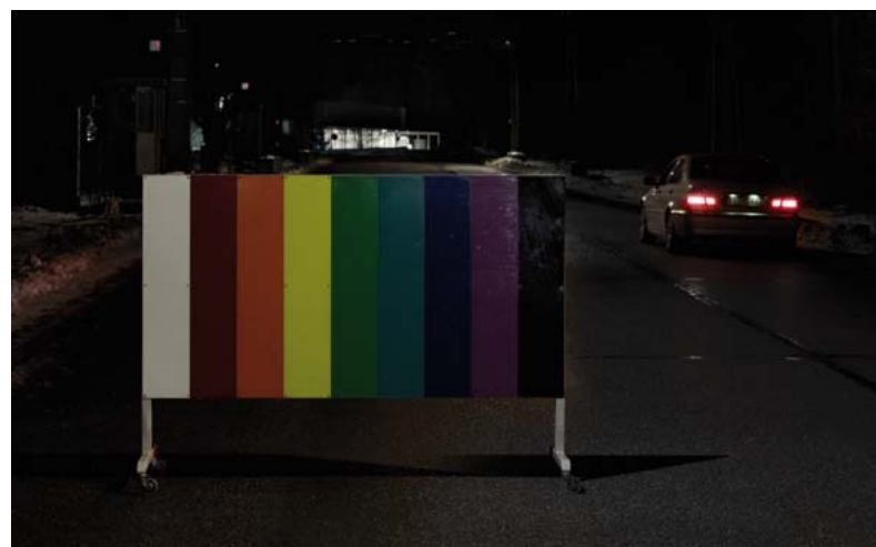
HME – road and environs have a blue-green tinge. Color rendering is limited. R_a 45-60
