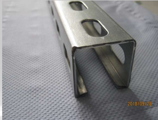
Element before testing in the salt chamber
