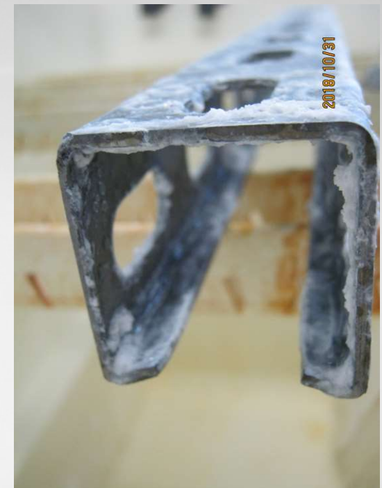
Element after 800 hours in the salt chamber
