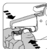
Squeeze wire stopper from both sides
