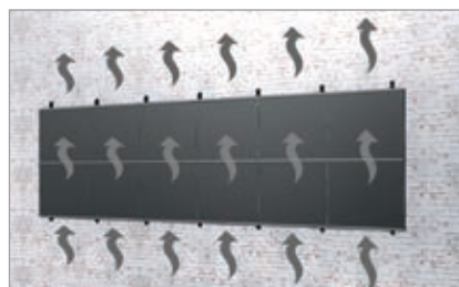
Very good rear ventilation of the modules
